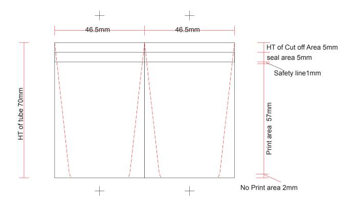
Dia. of tube: 30mm HT of tube: 70mm
